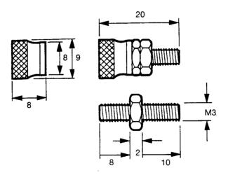
Uninsulated earthing post. A low cost uninsulated chassis mounting earthing post. Consist of a threaded section with a captive hex nut. Knurled fixing knob is not captive to enable use with ring terminals. Nickel plated brass construction.
